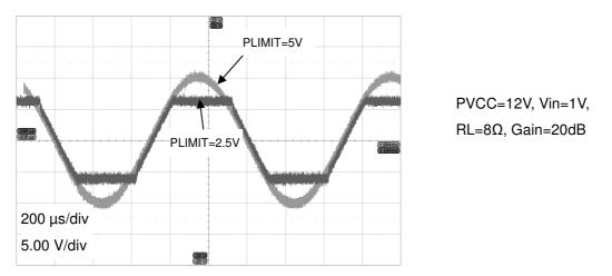
The PLIMIT circuit sets a limit on the output peak-to-peak voltage (waveform shown was recorded after passing through output low pass filters). The power clipping is done by limiting the duty cycle to a fixed maximum value converted from the voltage level at pin PLIMIT. This limit can be thought of as a "virtual" voltage rail which is lower than the supply voltage at PVCC. This "virtual" rail is around 2 times the voltage at the PLIMIT pin.
